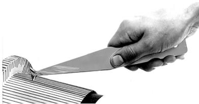
The Commutator Slot Shaver is a simple little hand tool to lightly chamfer the edges of commutator bars after undercutting. Pull it along the copper, shaving off the burs — flip it over and do the other edge.
