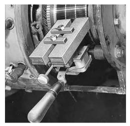
Type C mounted on Auxilliary Generator using only lower part of adjustable support.
