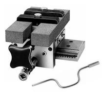
The "Comm-Pact" Grinding tool has a very low profile and is light-weight for use in confined spaces and on brush studs not heavy enough to support the weight of the large Commutator Grinder. Available in 6", 8", 10", and 12" lengths, each of which can grind up to 2" longer than its base length.
