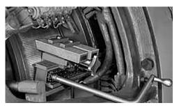
Grinder mounted on a Dieselelectric Generator
