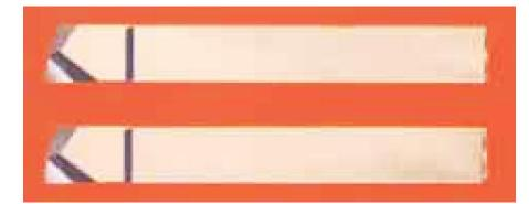
Diamond tipped turning tools shown are used in the finishing of the commutator surface. Steep rake angles on the tool ensure clean cutting of the copper, leaving no smearing or drag over across the mica. The nose radius of .010" leaves a very smooth surface to the copper requiring minimal preparation for the seating of brushes.
